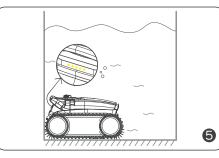
The device will automatically move to stop by the edge of wall when finishing cleaning or battery low.
