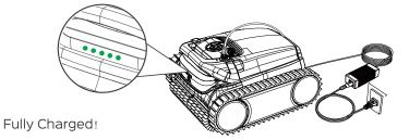
• For your important safety, you need to double check whether the device powers off and charging port is dry before charging.
