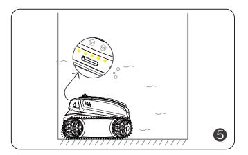
The device will automatically move to the docking station when finishing cleaning or battery is low.
