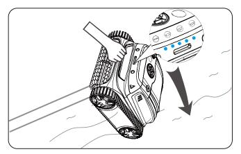
Turn on the device and put it into the pool vertically.
