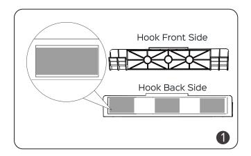
Take out three included adhensive gel nano tapes, and stick them onto the marked area on the station hook back side.
