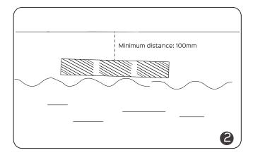
Find a flat wall 20mm above the waterline with a smoother surface and less dirt. Use a cloth to dry the surface. Ensure the area is not smaller than the hook.
