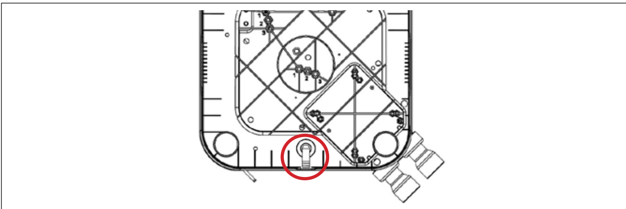
Condensate drainage orientation (seen from below the appliance)
