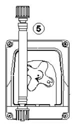
Insert the left hand fitting in the relative lodging and pass the tube beneath the roller's guide. Turn the probe holder in the direction of the circular arrow, while at the same time accompanying the tube into the head of the pump, until reaching the right hand fitting.
