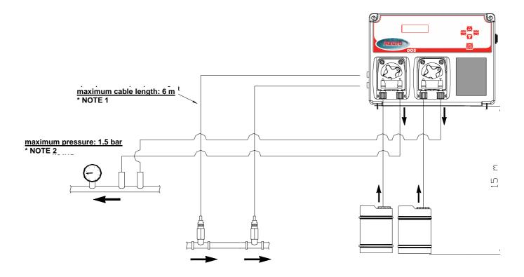
\* NOTE 1: IN ORDER TO AVOID ELECTRICAL DISTURBANCES, THE CABLE MUST PASS THROUGH A ZONE OTHER THAN THOSE USED FOR POWERING LARGE PUMPS.
