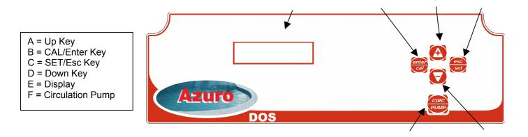
Press the **Down** and **SET** keys simultaneously to change the display mode. The two display modes are illustrated and described below:
