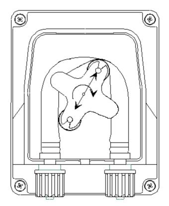
Before storing the regulation device, it is recommended to rinse the tube by pumping clean water.
