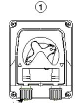
Release the cover by by pulling the left hand fitting upward.
