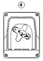
Position the roller at 10 and 20, turning it in the direction of the circular arrow.
