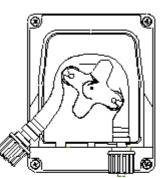
Completely release the fitting on the left, while continuing to press it outwards, and turn the roller in the direction indicated by the circular arrow so as to free the tube up until the right hand fitting.
